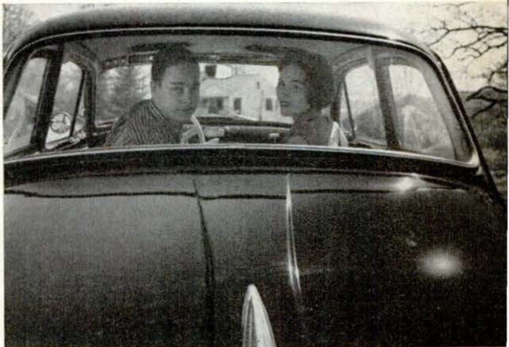
VISIBILITY to the rear is unusually good for a small foreign car. Safety-glass rear window is interchangeable with the windshield.
